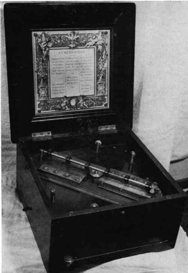
Left: the early Symphonion metal-disc-playing musical box. Note the two pairs of disc guide wheels and compare with the picture on page 153 of Volume 7. Above: the simple lever-wound motor and bedplate assembly with cylinder box-type governor. Below: star-wheel supports with combs removed showing inscription on single-drive dog turntable.
