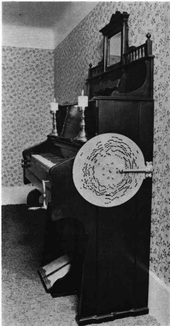
The view, left, shows the disc in position for mechanical playing. Unlike the Ariston mechanism, cranking the handle on the front of the organ serves only to rotate the music-disc. Suction must be created by pedalling at the same time to exhaust air from the reservoir seen in the view below. Above: looking down inside the organ with the complete top removed. The wire linkages from the keyframe (top of picture) to the 28 key actions of the mechanical player can be seen and their action evaluated from the patent drawing on page 6 which shows two alternative methods of admitting atmospheric pressure to the reeds so allowing them to be sounded.
