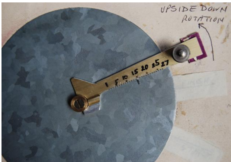
Figure 4 A blank disc fitted onto the jig with one projection put in place in one of the slots
