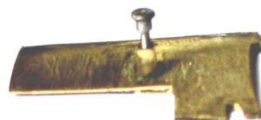
Figs 6 Little square pillars are soldered on the slides for starting and stopping
