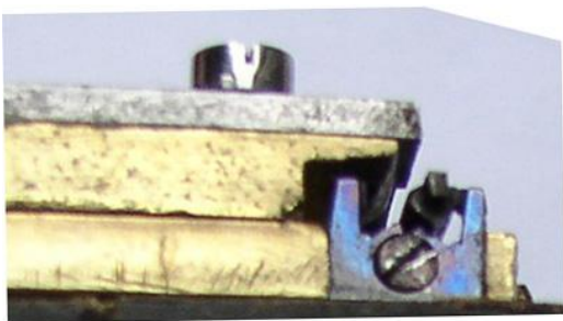
Fig 5 The change lever can be placed in three different positions
