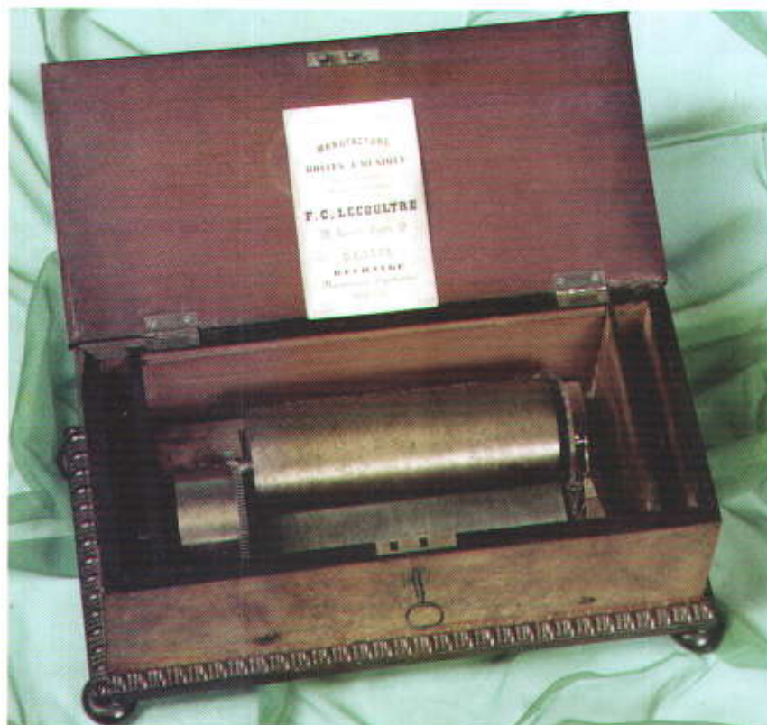
Interior of the F C Lecoultrre Overture Box revealing the large-diameter cylinder and the fine comb
