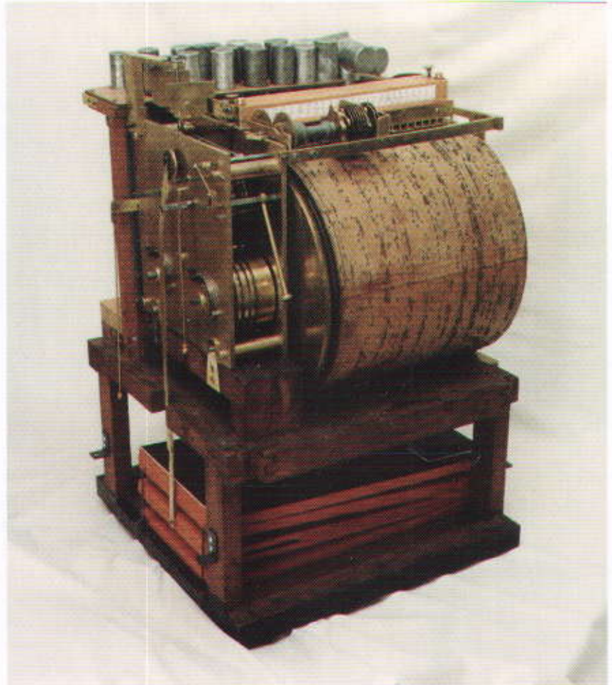
A quality organ mechanism by Alexandre Francois Debain of Paris. The large diameter wooden barrel shows that it plays fairly long melodies.
