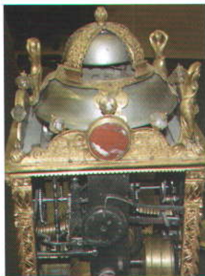
The locking plate for the strike mechanism together with details of the finely-decorated brasswork which mounts and partially contains the two striking bells. The main, larger bell is of a most curious cross-section while the strikework for the upper, smaller bell can just be seen under its rim.
