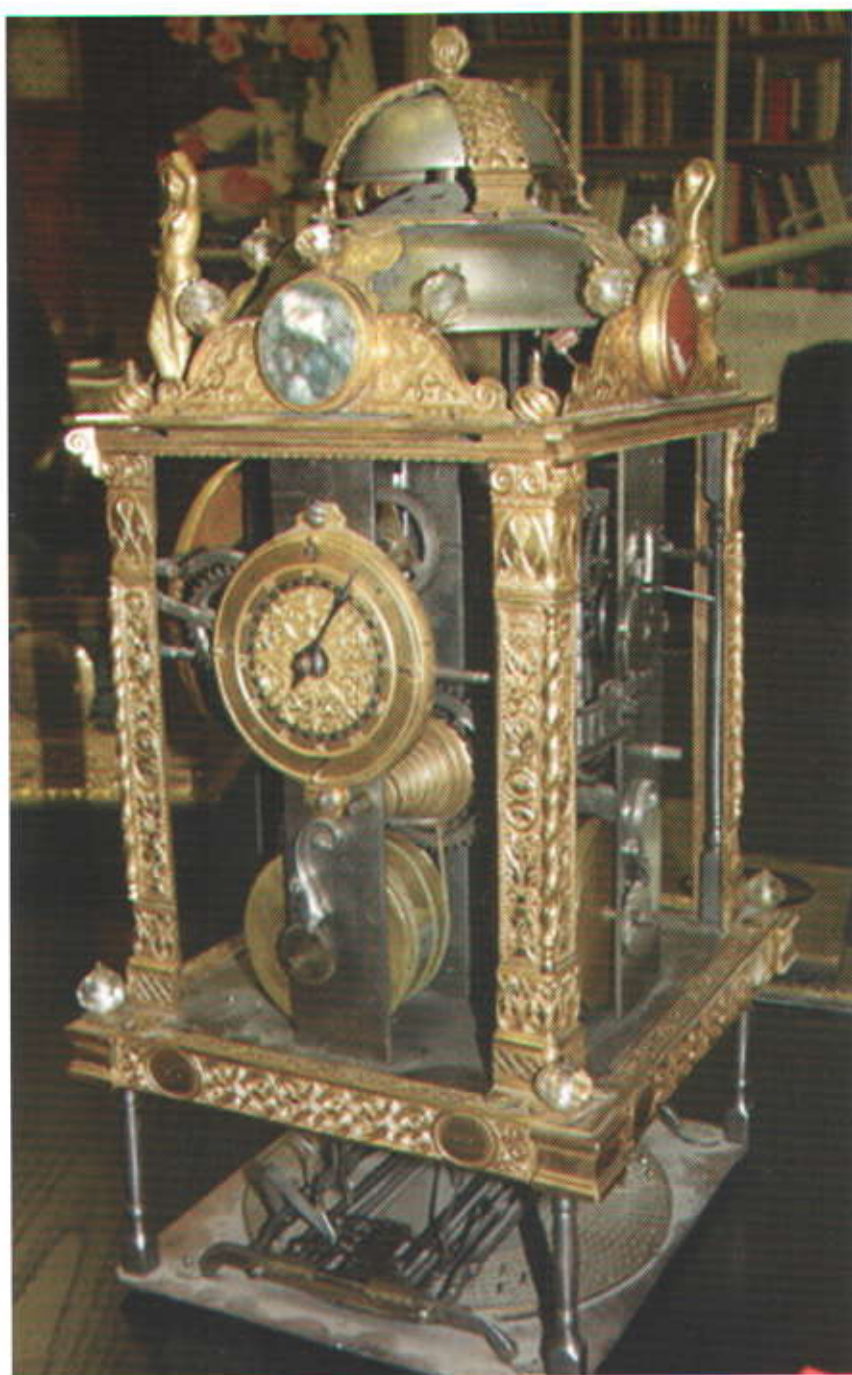
Lifting the whole clock clear of its base reveals this quite extraordinary and unique original musical mechanism that plays on eight bells arranged in a horizontal plane under the lower part of the clock proper.
