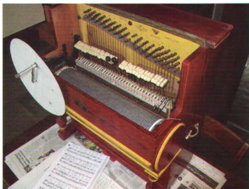
Cylinder with carbon paper and "clock face" attached, ready to be marked out. A bank of temporary coil springs hold the hammers away from the strings.
