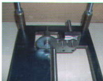
Fig 6. Bass end gears and transfer shaft take-off
