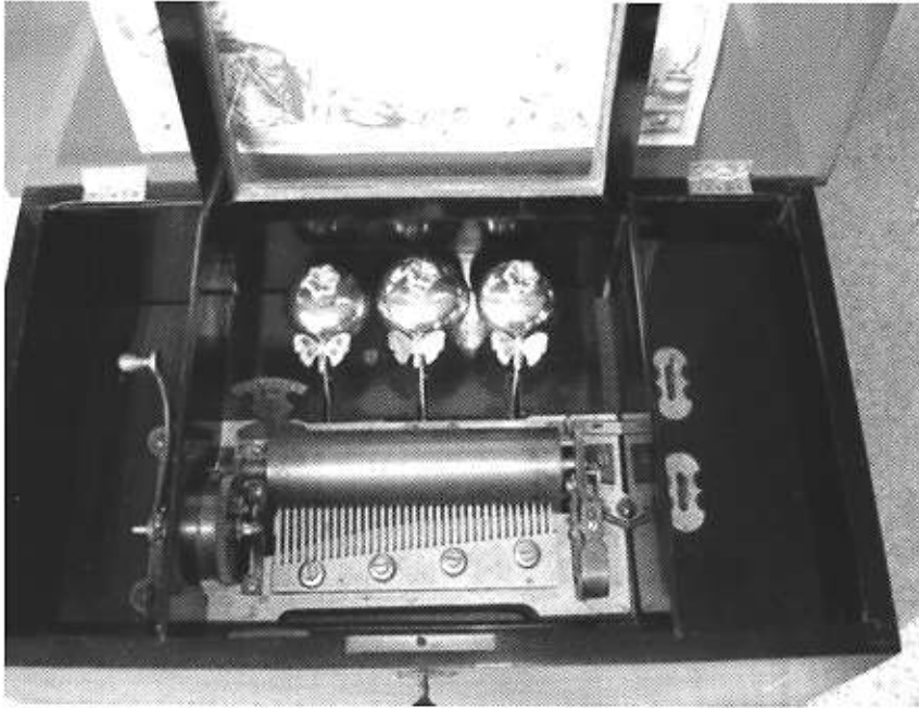
Three-bell box by B H Abrahams. Some examples have the outside bells playing simultaneously from a single comb tooth, so really they are two-bell boxes!
