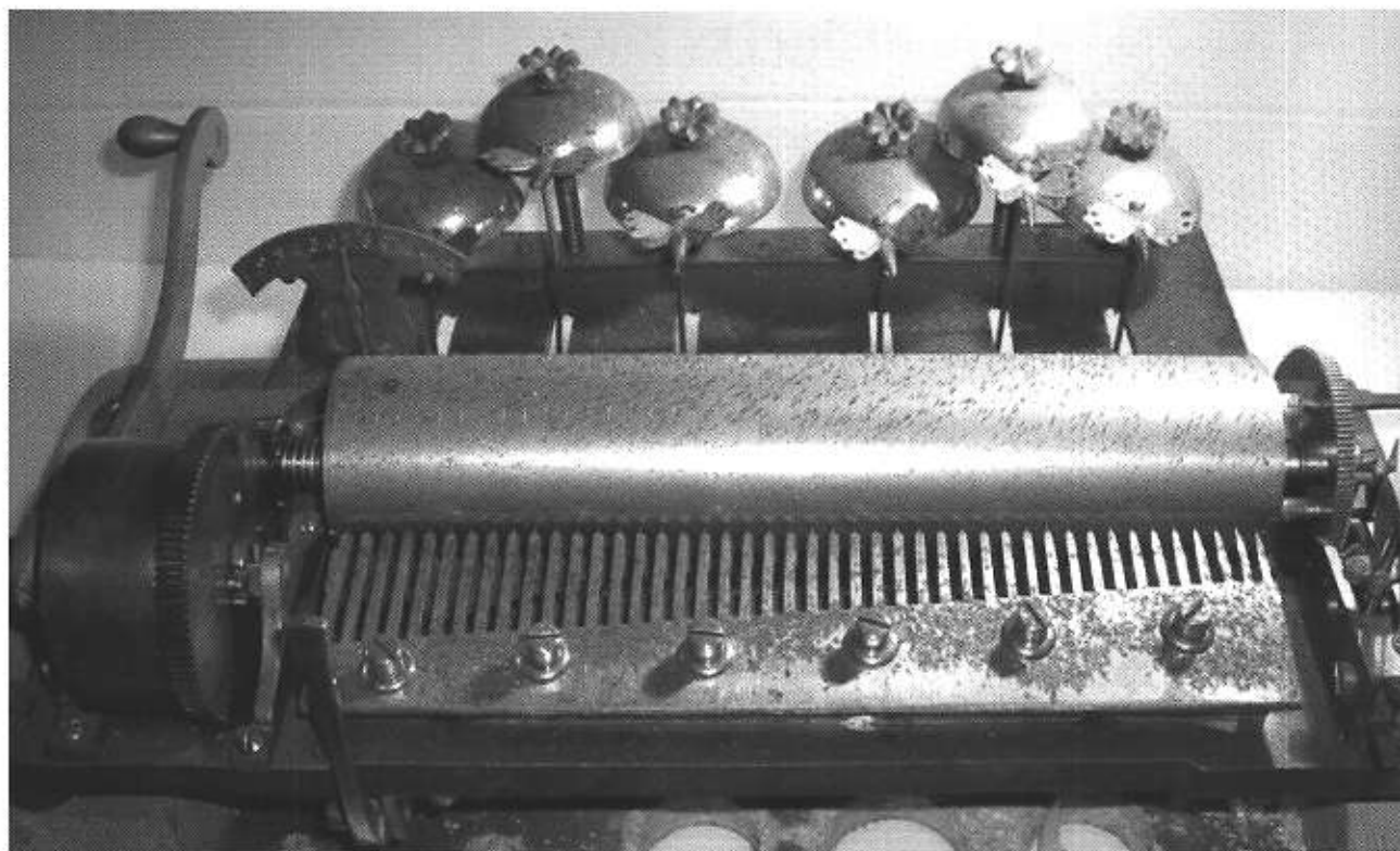
Unknown maker's late model 6-bell box with cheap plated steel bells, probably untuned. There appear to be only four bell teeth on the comb!
