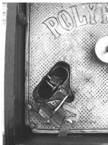
Photo 5: Polyphon 6.5 inch (16.4cm) - Detail View of Governor & Start-Stop Subassemblies
