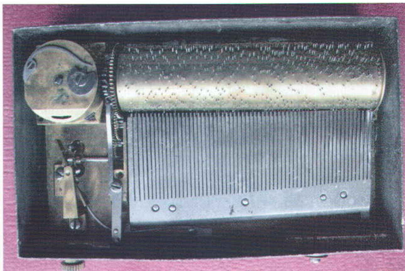
Below: Bill Cooper's unusual 'snuff box' movement in its tin box. Note the comb screws (upside down) and the unusual stop work. (Male part missing). See Letters page.
