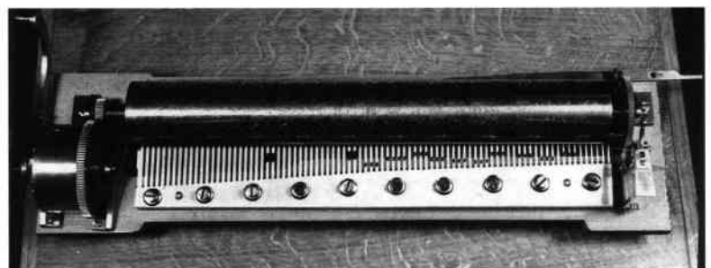
Fig.12 Mechanism of serial 3819 with the pairs of 440Hz and 880Hz a teeth marked, also the eight groups of 3 and one group of 4 teeth tuned to the same pitch.
